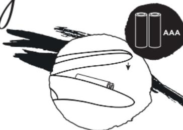
2. Take out the old batteries and give your ROMP some new life with new batteries. Watch out for +/- sign.
